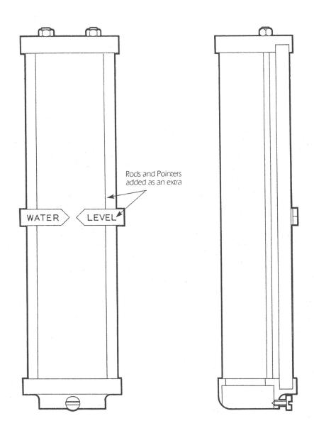
Top and Bottom Frames of Polished Cast Bronze. Best quality Toughened Plate Glass with Ground Edges.
